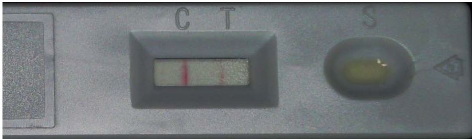
Reptest (Lateral Flow Cassette) showing two lines at 'C' and 'T' positions indicating positive for Fertility Associated Antigens (FAA)
