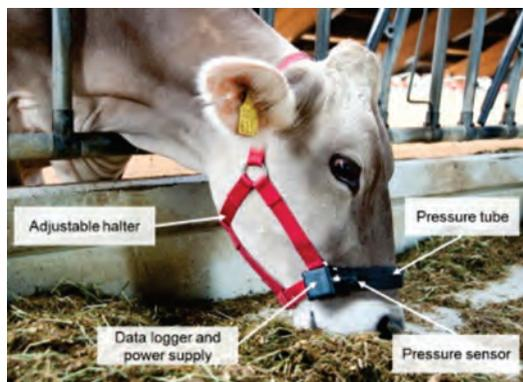
Fig. 4. Halter based device
