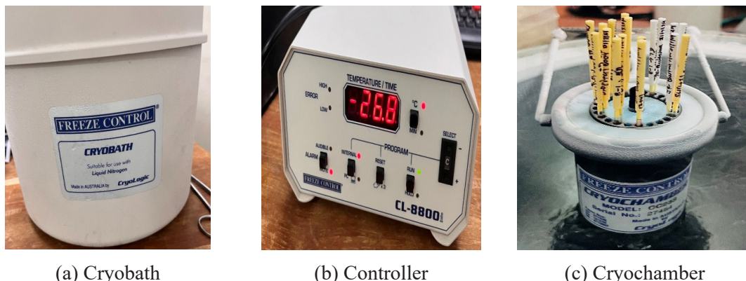
Fig. 1 Parts of Freeze Control by Cryologic for slow freezing of embryos
