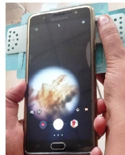
Figure 2: Foldscope attached with smartphone to visualize and click pictures of parasitic specimens.
